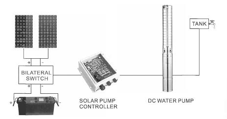
Solar photovoltaic panels convert sunlight energy to electricity energy through solar pump controller. The solar pump controller stabilize the voltage and creates a three phase output to drive the electric motor of the pump.
